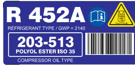
Figure 3. Refrigerant and Compressor Oil Nameplate
